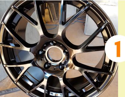
Single Stage Powders generally only require one coat or baking cycle
