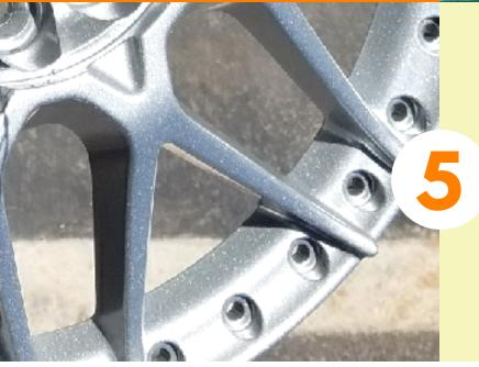
Metallics have varying levels of particulates for dazzle and shimmer there are single and two-stage applications
